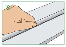
Fit inner sash, fit in parting bead (QW-CPB8) into clip profile (QW-SC1). Push and tap down until you hear the
