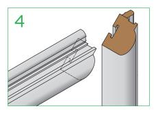
Measure sash frame and cut staff bead to size. Mitre cut top, bottom and side bead.
