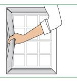
Bend centre of bead by hand and locate opposite end into clip profile at bottom corner mitre. Allow bead to snap back and tap down entire length until you hear the click. Repeat on other side.
