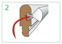
Cut parting bead to size. Slide seal (supplied separately) into finished parting bead (QW-CPB8).
